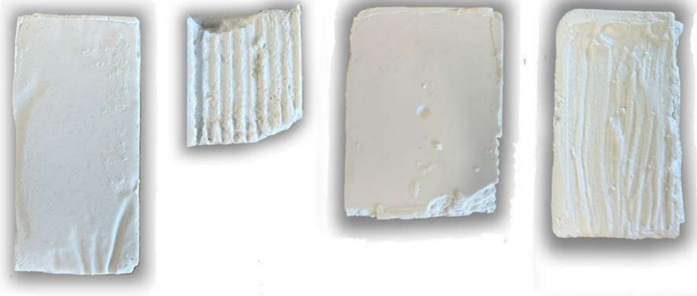
Tests with plaster casting in formwork, with different materials for different detailed finishes
