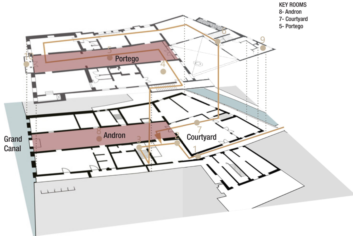
Figure 1 - The layout of Palazzo Vendramin Grimani | Visual by Zhutong Li | Group study by Cameron Linden Green, Srivinda Ladha, Zhutong Li.
